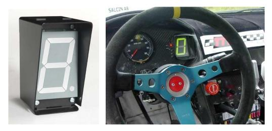
Part no. 10-031-5 Part no. 10-109-9 Display with cablekit Sunvisor and mountingkit
