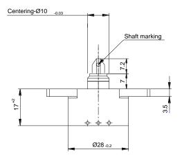
When the shaft marking is pointing to terminal 2 (red), the wiper is located in an electrical center position.
